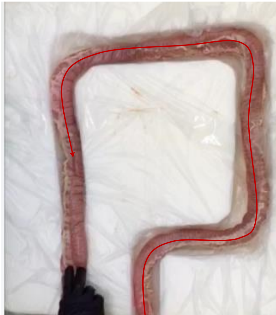
Figure 4 - 3: Benchtop test of colonoscopy robot in an excised porcine colon.
