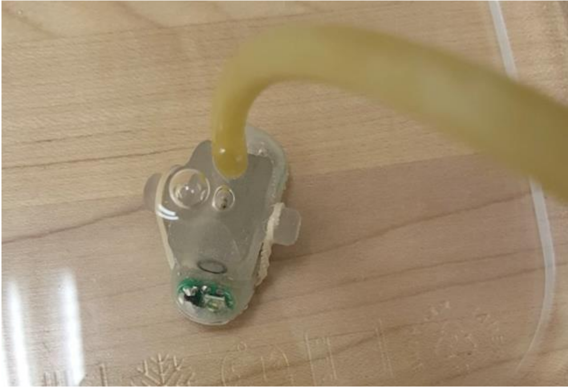
Figure 7 - 2: Blow test device
