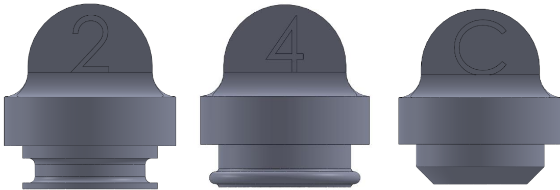
Figure 7 - 4: Plugs representing sensor plate seal geometry
